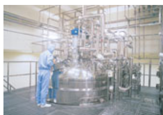
Antibody production cell culture: Cells are transplanted into a 10,000-liter bioreactor for cultivation.
